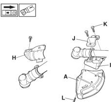
Remove the mounting plate (H). Fit the adapter (I) and bracket (J) with the two screws (K) as shown. Fit the blade guard (A) to the adapter using the 4 screws (L) as shown.
